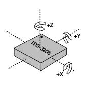
Orientation of Axes of Sensitivity and Polarity of Rotation
