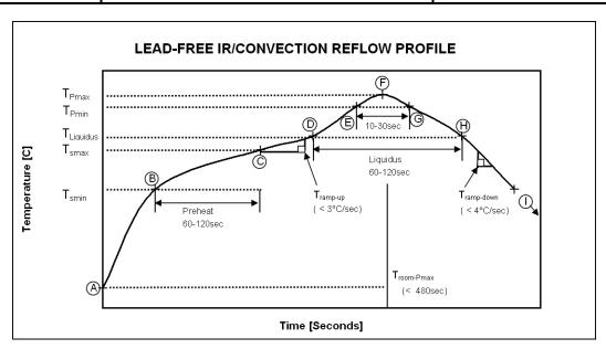
Maximum Temperature IR / Convection Solder Reflow Curve Used for Qualification
