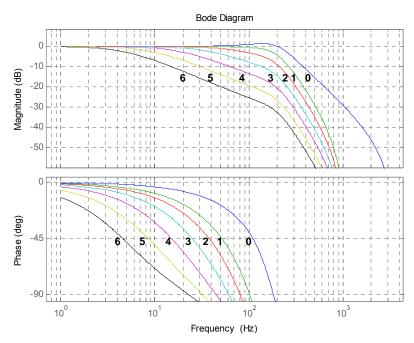
Gain and Phase vs. Digital Filter Setting
